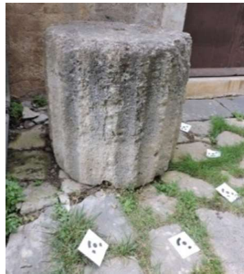
Fig. 5. Targets were placed around the drum S1 during the capturing process.
