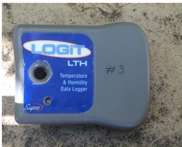
Fig. 2: Fixed temperature, humidity logger
